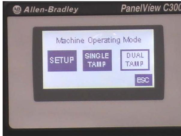
Note: Prior to changing Timers in the individual save areas, select the applicable mode (single or double tamp) that will be adjusted. For example, if the Single Tamp is selected and then timers are changed in the Dual Tamp save areas, the changes will not be saved.
