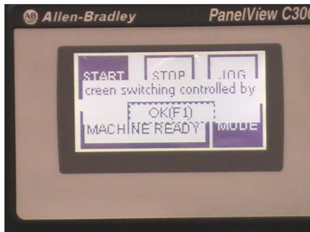
Depressing the OK (F1) button will clear this screen and return it back to the main screen. Remember, always go to the Stop button first prior to going to another function. Once back to the
