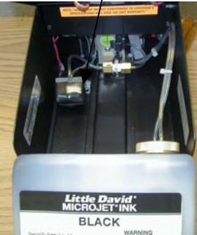
Reservoir in Purge Position
