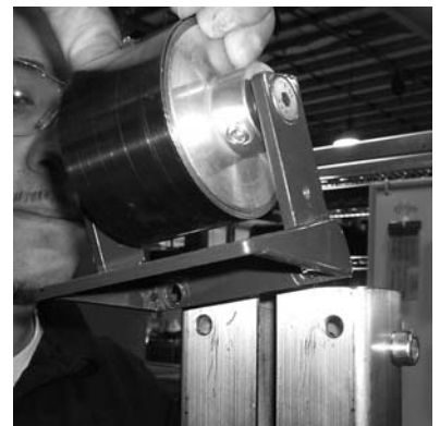
Figure 5: Remove spring bracket assembly from top of mast.
